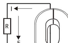
loop. The Meter will measure E & I, and the measured resistance R can be obtained by the following formula.
