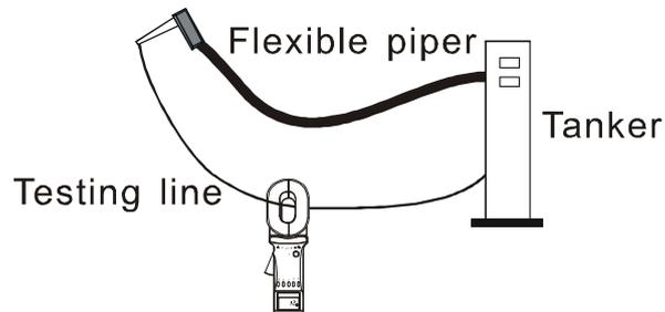
Connect Fuel truck nozzle and tanker by one testing line. Read  $R_T$  by meter, then can figure out: the connect resistance of oil transmission piper of tanker:  $R=R_T-R_L$
