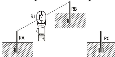
Second, have  $R_B$  and  $R_C$  linked up, as shown in the following figure. Use the Meter to get the second reading  $R_2$ .
