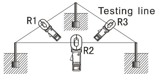
Tanker grounding pole A Auxiliary grounding pole B Grounding pole C of upload and load place
