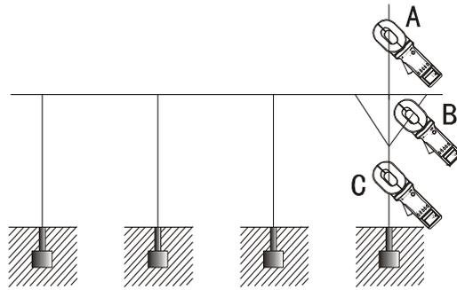
When measuring at A point, the branch doesn't form a circuit, the meter shows "OL Ω", then should change the measuring point.
