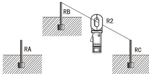
Third, have  $R_C$  and  $R_A$  linked up, as shown in the following figure. Use the Meter to get the third reading  $R_3$ .
