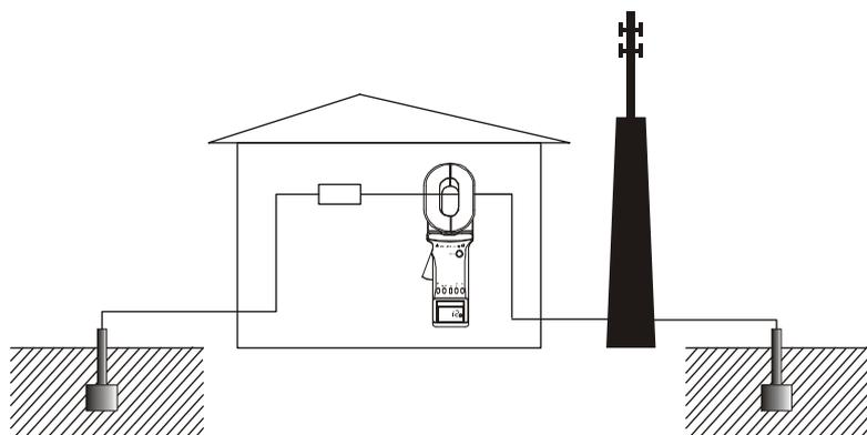
If the value of meter is lower than the allowable value of grounding resistance, then the grounding resistance of machine room and the launch tower is valid. If the value is greater than allowable value, please measure by single point grounding method.
